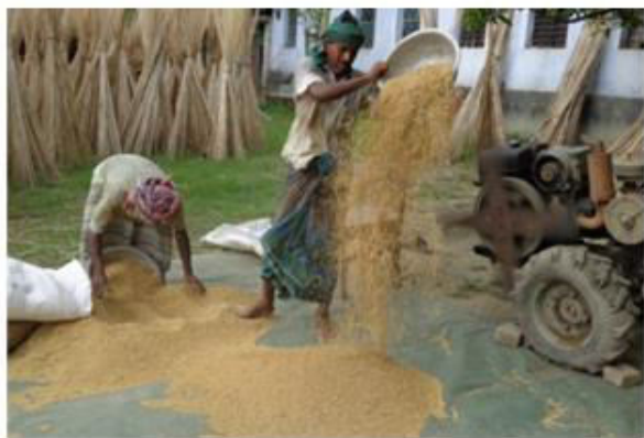
Fig. 7: PT operated grain cleaner without safety cover tested in farmer’s yard.
